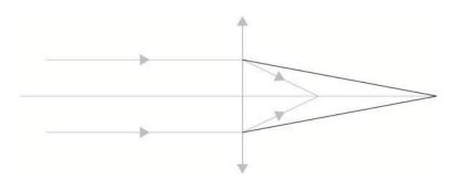
the refracted rays converge on the principal axis farther from the lens than for blue;
